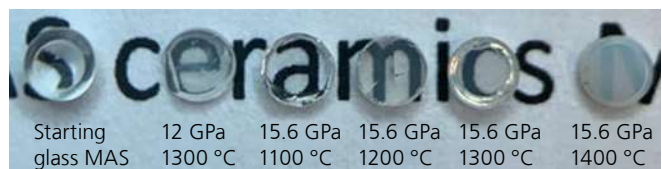
Fig. 3: Transparent ceramics produced via the high-pressure route at different pressures and temperatures, diameter approx. 3–5 mm.
